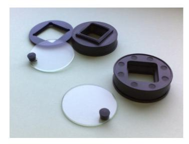
The CYTOOchamber™ is a 35mm footprint device specially designed and manufactured for our 2x2cm² square CYTOOchip™ format which enables you to do high resolution timelapse microscopy.
