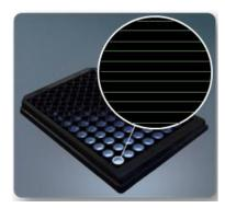
CYTOOplates *Motility* are glass-bottom microplates, bearing arrays of adhesive lines in each well. Each CYTOOplate offers 4 different line widths for 1D cell migration (2.5, 5, 10 and 20  $\mu$ m), with a line-to-line gap of 45  $\mu$ m.
