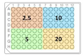
**24** identical wells per zone Well diameter: 6.3 mm
